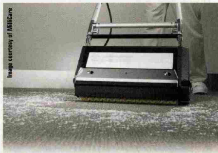
With dry compound cleaning, carpets are cleaned without the use of water, an increasingly popular option in drought-stricken regions.
